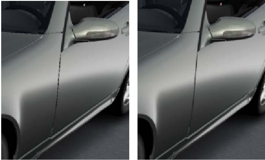
Figure 3. The image on the left uses a regular multisample pattern; the image on the right uses a rotated multisample pattern.
