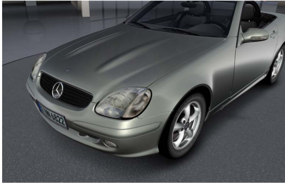
Figure 5. Unmagnified screen capture from an automotive styling application, showing the superior visual quality of multisampling using a rotated grid.
