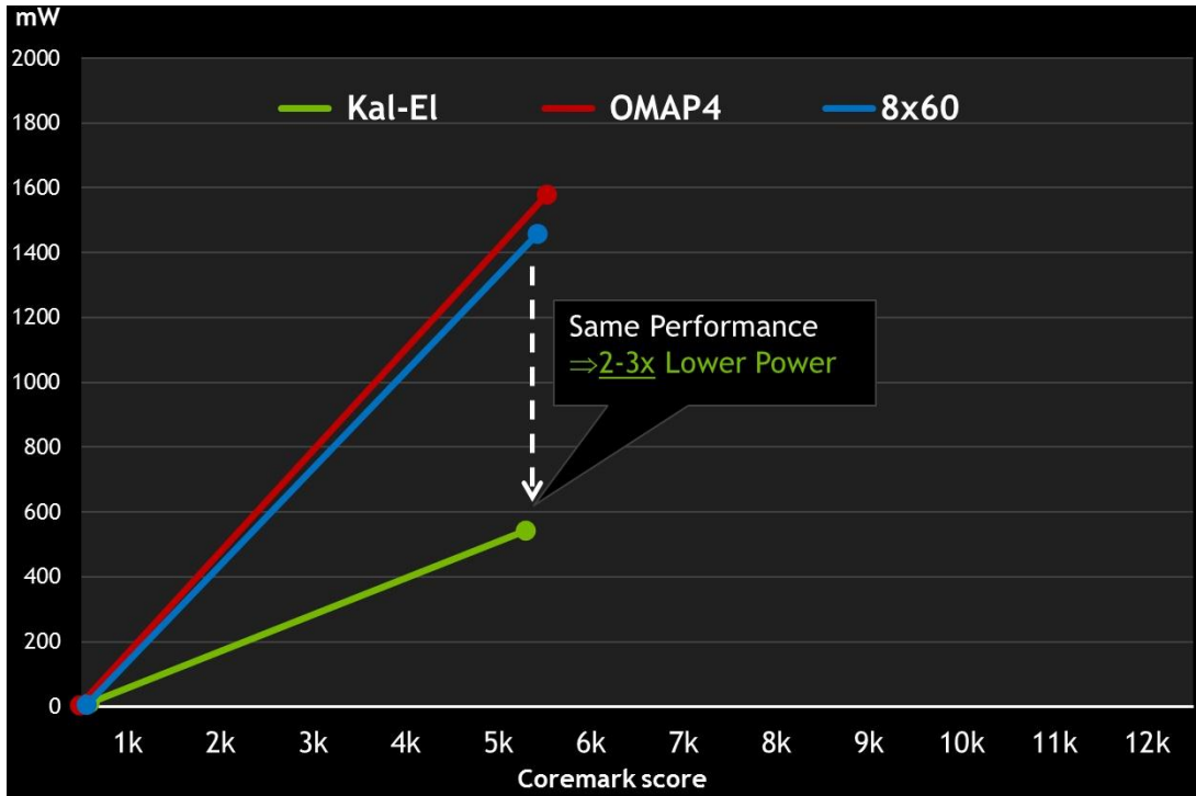
Figure 7 Kal-EI power consumption when delivering the same performance as competing dual core processors
