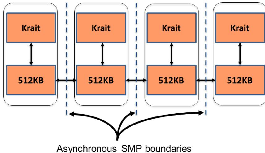
**Figure 8 Asynchronous SMP prevents Krait from allocating the entire L2 to a single CPU core**
