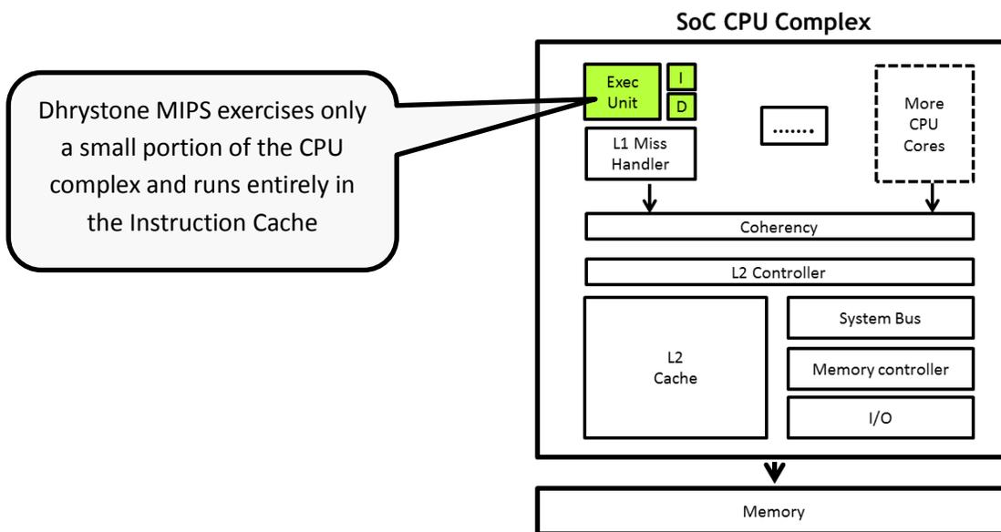
Figure 2 Dhrystone MIPS benchmarks only a small section of the CPU complex
