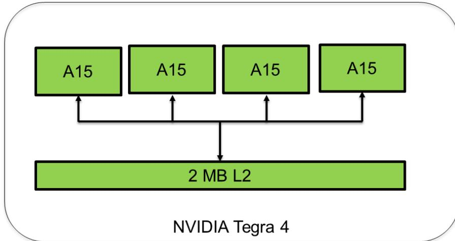
**Figure 7 Entire 2MB L2 cache can be dynamically allocated to any CPU on NVIDIA Tegra 4**
