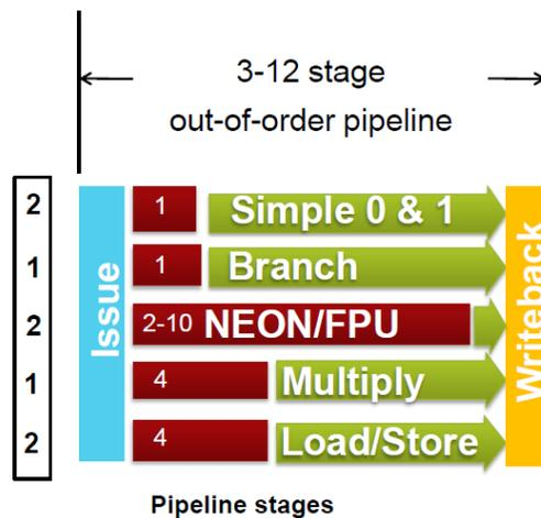
Figure 4 Eight Execution Units on ARM Cortex-A15 CPU
