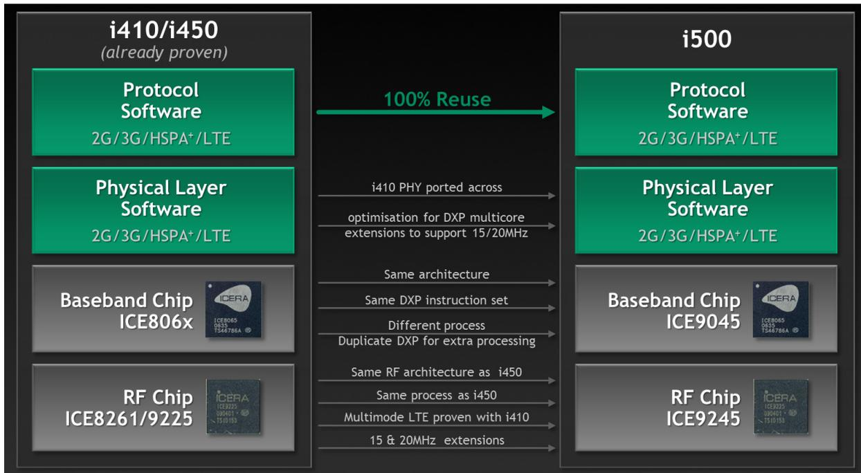
Figure 5 Significant reuse of LTE Multimode software from 4<sup>th</sup> generation NVIDIA modem
